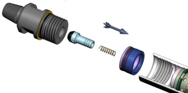
9. Check the backhead compression gap. This gap is critical for keeping the internal parts tight.
