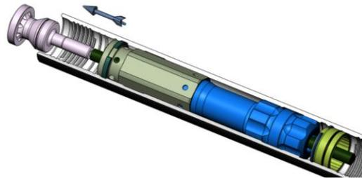
7. Remove the cylinder and piston. Stand the sleeve on the backhead end. The piston will drop against the cylinder. Using a rod, pipe, or timber (3" dia max x 40" long) and a sledge hammer, or just a heavy bar (Rock Hog uses a 2-1/2" dia x 5' long steel bar), drive on the piston. This will collapse the ring out of its groove and allow the cylinder and piston to move to the bottom of the sleeve. Lay the sleeve over and push the cylinder/piston out of the sleeve.
