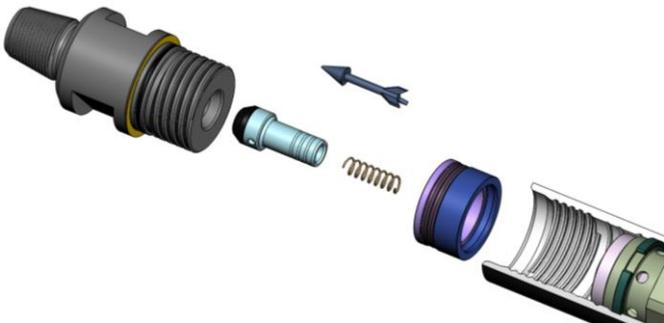
4. If the disc springs look dry and/or rusty, pull the disc spring pack apart. The guide ring is held inside the spacer tube by an o-ring. Hold the spacer tube and tap the guide ring out, remove the o-ring, slide the disc springs off the ring.
