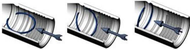
3. Set in the bit retainer ring (NOTE: the ring is not symmetrical, the o-ring end must be toward the chuck). If used, put the breakout washer on the chuck and thread in the chuck. The chuck should seat up on the sleeve. If there is a gap, parts are out of place. Find the cause of the gap and correct it.
