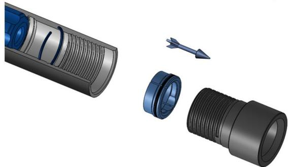
6. Drive out the air distributor from the chuck end with a steel rod or pipe (7/8" max dia x 30" min long). run the rod through the piston to push out the air distributor.
