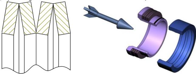
Set disc spring pack, spacer down, on top of the air distributor.
