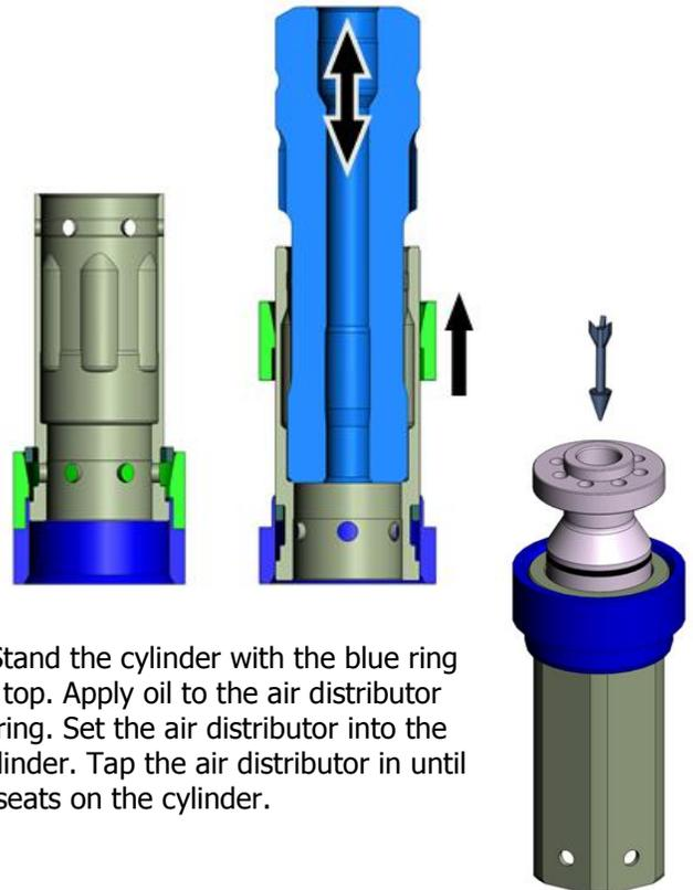
Stand the cylinder with the blue ring at top. Apply oil to the air distributor o-ring. Set the air distributor into the cylinder. Tap the air distributor in until it seats on the cylinder.
