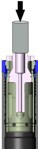
The ring will only seat into the correct location so drive the cylinder in until it comes to a hard stop. The top of the air dist will be below the sleeve 5.64" (143mm). Remove the blue ring and driver from the sleeve.
