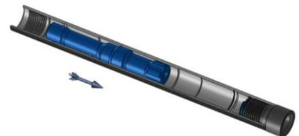
6. Install the cylinder/air distributor next: stand the hammer, chuck down, on a solid surface. Set the cylinder into the sleeve. Push/tap it in until the blue ring seats on the sleeve. Place a piece of soft steel, aluminum, or wood on top of the air distributor (*Rock Hog uses a piece of aluminum 2.5" round X 6" long*). With a sledge hammer, drive the cylinder/air distributor into the sleeve.
