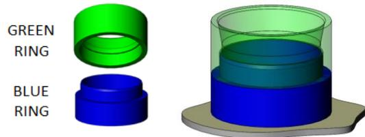
Set the cylinder into the ring stack, then set the piston down into the cylinder. Using the piston as a bump hammer, drive the cylinder into the ring stack until the cylinder hits the surface (*a few high-force blows with the piston work best*). Now pull the piston out of and slide the green ring off of the cylinder. The blue ring will stay on the cylinder keeping the cylinder retainer ring collapsed in the cylinder groove.
