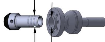
Clearance may be checked using feeler gages or by measuring both parts with micrometers. Additional details are given under individual parts below. Again, keeping a log of when & what service was performed will help fine-tune the service schedule to fit your operation.
