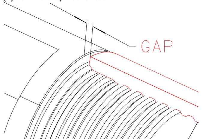
10. Once the gap is correct, remove the backhead, put the breakout washer on if used and put the o-ring on. Apply thick coating of copper coat grease to the backhead wear sleeve threads. Turn the backhead into the sleeve until hand tight. If available, put a thread protector cap on the drill pipe thread.
