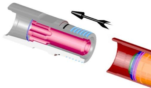
5. Lift out the check valve, check valve spring, washer and (3) disc springs.
