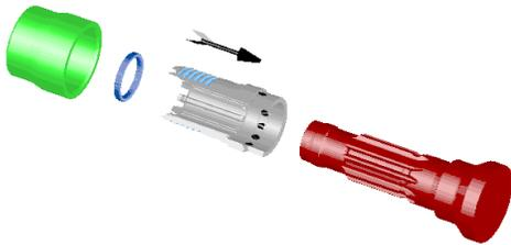
Thread the chuck back into the wear sleeve. The shroud will seat right onto the sleeve. There should be no gap.
