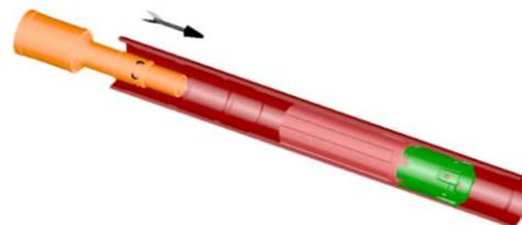
7. Set in the disc springs. Make sure the bevel on the springs alternate.
