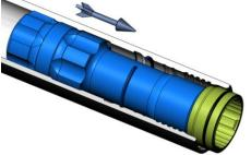
b. Pull method: (*This will allow the piston to be removed from the chuck end if the backhead is still tight*). Prepare a bump-out hammer from these parts:
