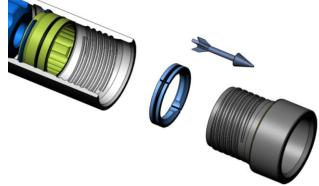
6. Drive out the air distributor from the chuck end with a steel rod or pipe  $(1-1/8'' \max \text{ dia } x \ 30'' \min \text{ long})$ . Run the rod through the piston to push out the air distributor.
