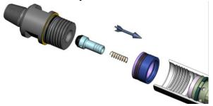
10. Check the backhead compression gap. This gap is critical for keeping the internal parts tight.
