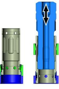
Stand the cylinder with the blue ring at top. Apply oil to the air distributor o-ring. Set the air distributor into the cylinder. Tap the air distributor in until it seats on the cylinder.
