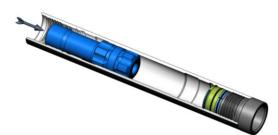
7. Install the cylinder/air distributor next: stand the hammer, chuck down, on a solid surface. Set the cylinder into the sleeve. Push/tap it in until the blue ring seats on the sleeve. Place a piece of soft steel, aluminum, or wood on top of the air distributor (*Rock Hog uses a piece of aluminum 2.5" round X 6" long*). With a sledge hammer, drive the cylinder/air distributor into the sleeve.
