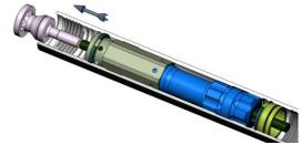
7. Remove the cylinder and piston. Stand the sleeve on the backhead end. The piston will drop against the cylinder. Using a rod, pipe, or timber (2-7/8" dia max x 40" long) and a sledge hammer, or just a heavy bar (*Rock Hog uses a 2-1/2" dia x 5' long steel bar*), drive down on the piston. This will collapse the ring out of its groove and allow the cylinder and piston to move to the bottom of the sleeve. Lay the sleeve over and push the cylinder/piston out of the sleeve.
