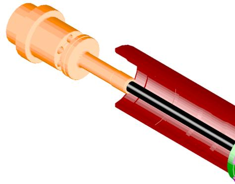
8. Remove the piston & cylinder. Stand the sleeve on the backhead end on a solid surface. With a heavy rod or timber on the piston face, drive on the piston (Rock Hog uses a 2-1/2" diameter X 60" long steel bar). The cylinder is held in by a retaining ring that will collapse out of its groove allowing the parts to come out. It will take moderate force to collapse the ring. Once collapsed, the parts will advance with less force. Drive the parts down until they hit bottom
