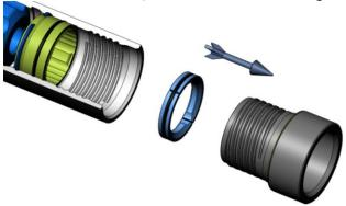
6. Drive out the air distributor from the chuck end with a steel rod or pipe (1-1/2" max dia x 30" min long). Run the rod through the piston to push out the air distributor.
