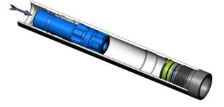
7. Install the cylinder/air distributor next: stand the hammer, chuck down, on a solid surface. Set the cylinder into the sleeve. Push/tap it in until the blue ring seats on the sleeve. Place a piece of soft steel, aluminum, or wood on top of the air distributor (*Rock Hog uses a piece of aluminum 2.5" round X 6" long*). With a sledge hammer, drive the cylinder/air distributor into the sleeve.
