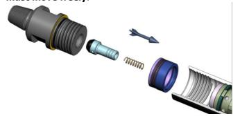
10. Check the backhead compression gap. This gap is critical for keeping the internal parts tight.
