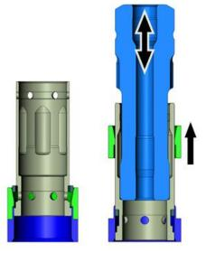
Stand the cylinder with the blue ring at top. Apply oil to the air distributor o-ring. Set the air distributor into the cylinder. Tap the air distributor in until it seats on the cylinder.
