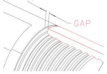
11. Once the gap is correct, remove the backhead, put the breakout washer on if used and put the o-ring on. Apply thick coating of copper coat grease to the backhead wear sleeve threads. Turn the backhead into the sleeve until hand tight. If available, put a thread protector cap on the drill pipe thread.
