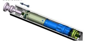
7. Remove the cylinder and piston. Stand the sleeve on the backhead end. The piston will drop against the cylinder. Using a rod, pipe, or timber (2-1/2 dia x 40" long) and a sledge hammer, or just a heavy bar (*Rock Hog uses a 2-1/2" dia x 5' long steel bar*), drive down on the piston. This will collapse the ring out of its groove and allow the cylinder and piston to move to the bottom of the sleeve. Lay the sleeve over and push the cylinder/piston out of the sleeve.
