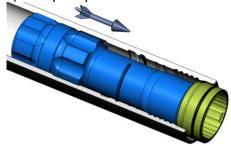
b. pull method: (this will allow the piston to be removed from the chuck end if the backhead is still tight) prepare a bump-out hammer from these parts: +Block- 1/2 x 1-1/2 x 3-3/16 x 3-1/4 across corners, with a threaded center hole,
