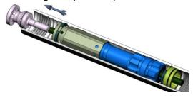
7. Remove the cylinder and piston. Stand the sleeve on the backhead end. The piston will drop against the cylinder. Using a rod, pipe, or timber (2-3/4" dia x 40" long) and a sledge hammer, or just a heavy bar (*Rock Hog uses a 2-1/2" dia x 5' long steel bar*), drive down on the piston. This will collapse the ring out of its groove and allow the cylinder and piston to move to the bottom of the sleeve. Lay the sleeve over and push the cylinder/piston out of the sleeve.
