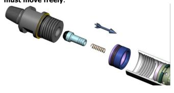
10. Check the backhead compression gap. This gap is critical for keeping the internal parts tight.
