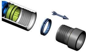
6. Drive out the air distributor from the chuck end with a steel rod or pipe (1" max dia x 30" min long). Run the rod through the piston to push out the air distributor.
