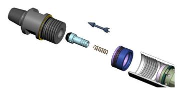
4. If the disc springs look dry and/or rusty, pull the disc spring pack apart. The guide ring is held inside the spacer tube by an o-ring. Hold the spacer tube and tap the guide ring out, remove the o-ring, slide the disc springs off the ring.
